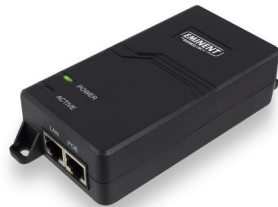
ActivePoE Automatic Power Negotiation GigabitEthernet Connections Max30Watt IEEE 802.3af/at compliant
