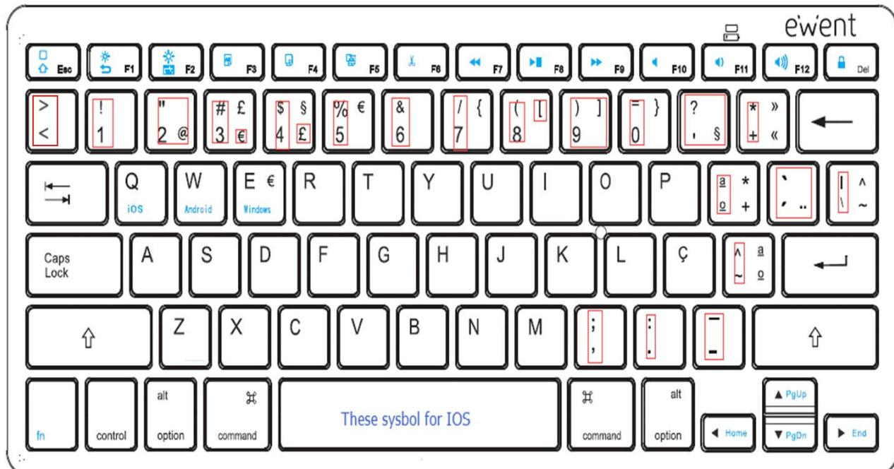
Keys Android - USE "FN" KEY + "W" FOR OPERATING IN ANDROID
